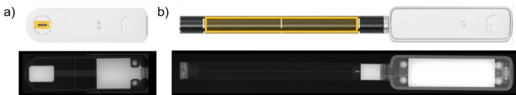
**Figure 2: The active sensor areas and corresponding radiological footprints of the X2 R/F and the X2 CT. a)** The X2 R/F has an active sensor area of 0.4 cm x 0.9 cm (yellow). The diodes and the electronics part of the sensor are shielded with tin (light areas in X-ray image). **b)** The X2 CT has an active sensor area of 10 cm x 1 cm (yellow) that is virtually transparent to X-rays. The electronics part of the sensor is shielded with tin (light areas in X-ray image).
