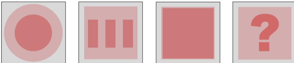
**Figure 1:** Top-down view from the X-ray source with examples of different AEC/ABC areas (dark red) on the total irradiated area (light red).
