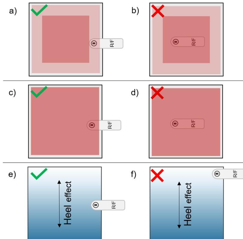
**Figure 4: Positioning of the X2 R/F for measurements on X-ray systems with AEC/ABC. Top-down view from the X-ray source with primary X-ray radiation in light red and AEC area of the machine in darker red. Heel effect depicted in blue.**
