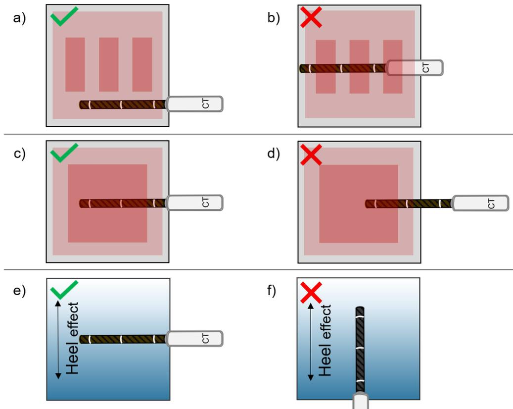
**Figure 5: Positioning of the X2 CT for measurements on X-ray systems with AEC/ABC. Top-down view from the X-ray source with primary X-ray radiation in light red and AEC area of the machine in darker red. Heel effect depicted in blue.**
