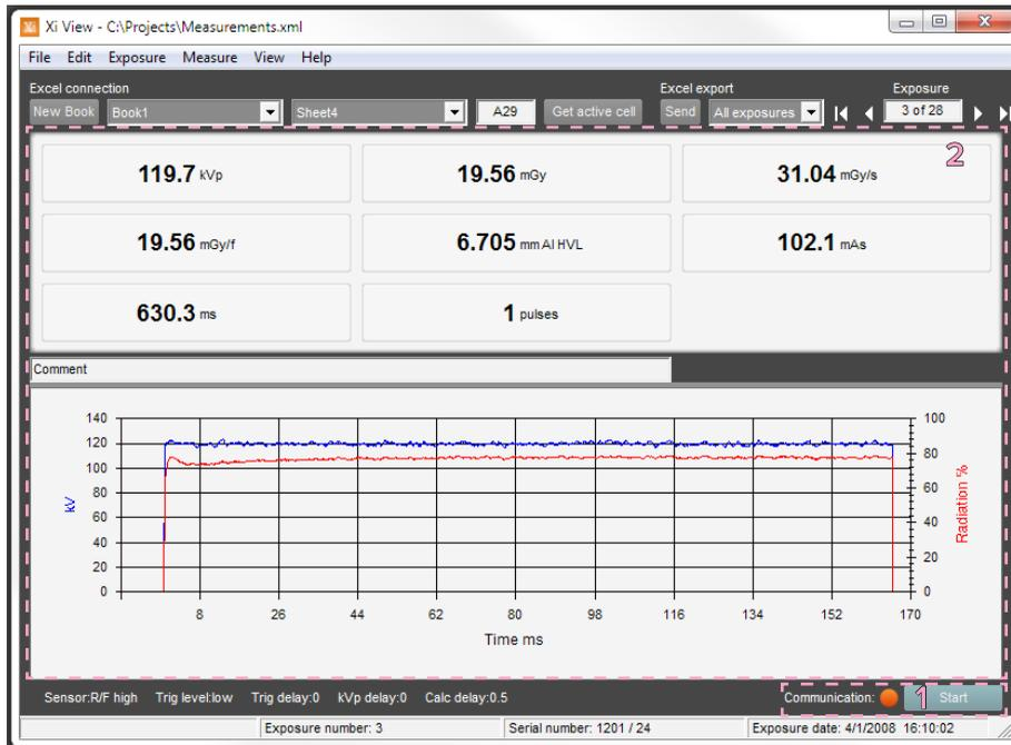
Figure 2. RaySafe Xi View main window.
